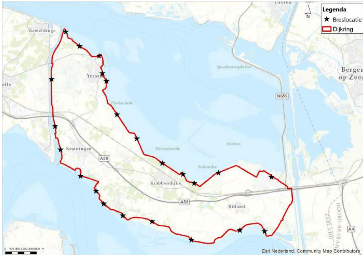
Figure 2.2 Breach locations in the municipality of Reimerswaal
