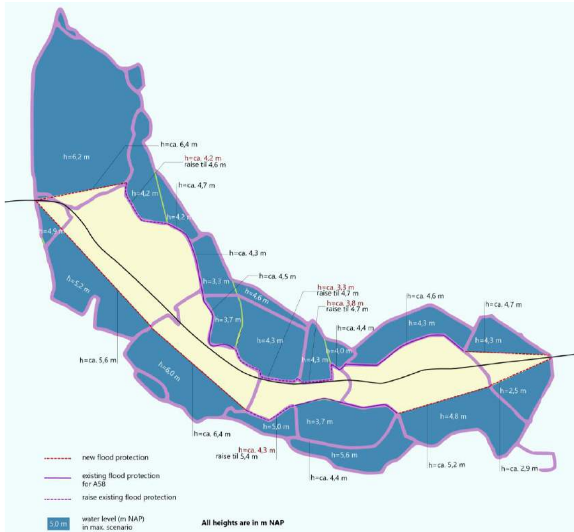
Figure 5.3 Continued functioning of A58 through compartmentalisation
