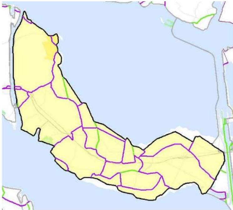
Figure 2.1 Purple: inner dyke with water management function, green: inner dyke without water management function (source: VNK2 report 'Flood risk Dyke Ring 31 South-Beveland', December 2011)
