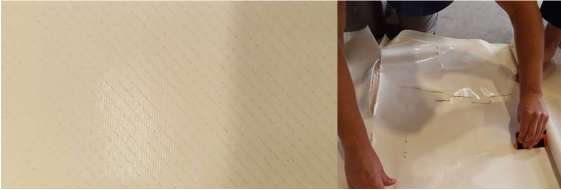
Figure 53: Left: Zoom-in of the fouling layer on the scale guard membrane (15/07/2021). Right: scraping of the fouling on the membrane.
