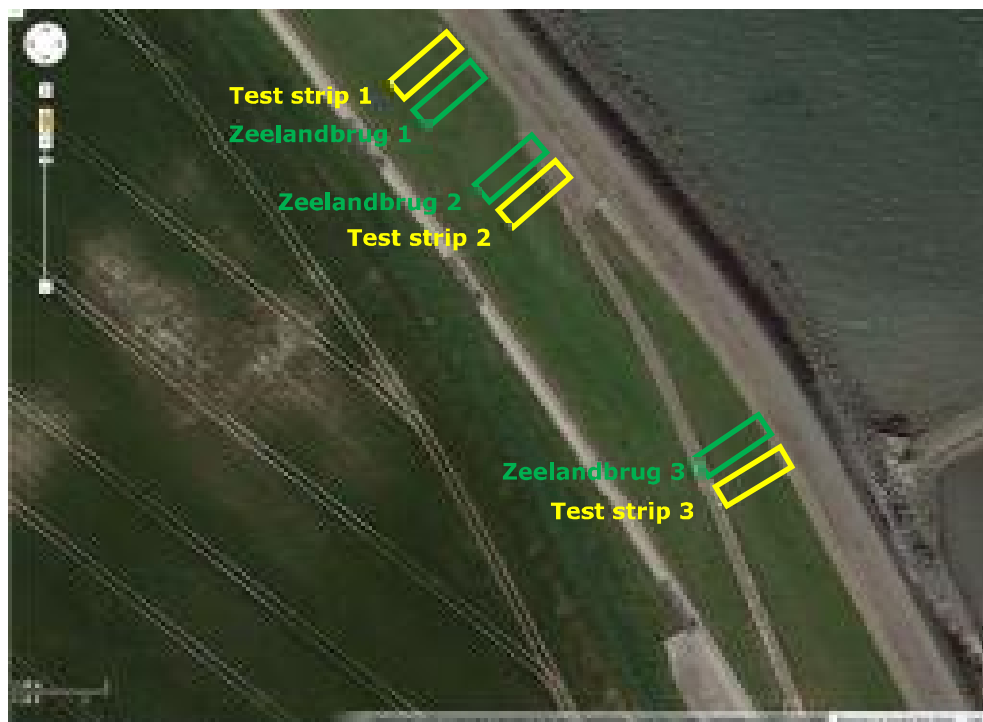
Figure 2: Detail of the test location. The yellow frames show the approximate locations of test strips for the wave run-up experiments. The green frames show the approximate locations of the sampling strips for sod quality measurements carried out by Alterra ('Zeelandbrug 1-3').
