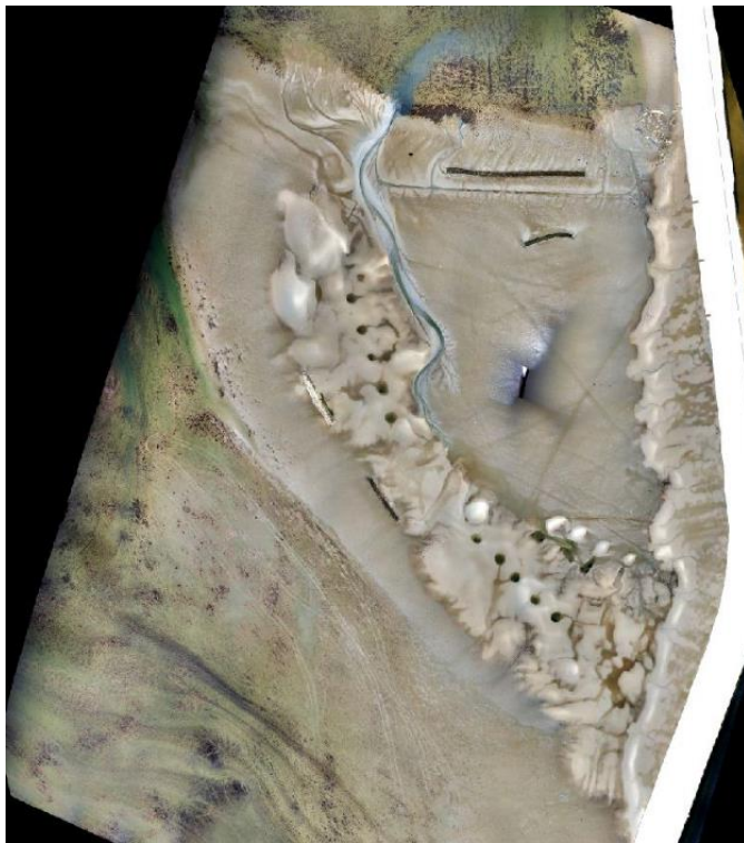
Figure 5-9. Orthogonal image of the Oesterdam sand nourishment at May 2014, image is created with a large number of photos taken by a drone.
