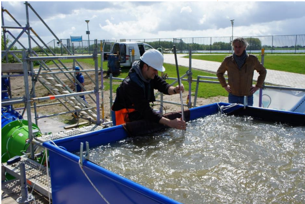
Figure 25. Measuring the water flow coming out of the large pipe with a Flow Mate 2000
