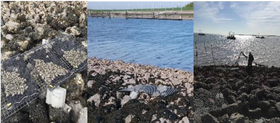
Figure 11. Oyster sacks were placed at two heights and at two levels of hydrodynamics at Goese Sas. Oyster sacks as attached to the steel sheet (left), placed low on the kreukelberm (70% inundation time) on the low hydrodynamic side of the breakwater (middle), and high on the kreukelberm (50% inundation time) on the high hydrodynamic side of the breakwater (right).
