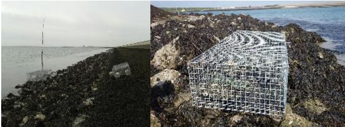
Figure 10. Oyster sacks were placed in steel gabions at two heights and at two levels of hydrodynamics at De Schelphoek. Oyster sacks as placed at both heights (low for 70% inundation time and high for 50% inundation time) on the low hydrodynamic side of the breakwater (left), and on the high hydrodynamic side of the breakwater (right).
