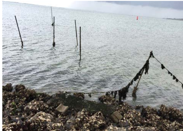
Figure 12. While the mesh sheet and concrete blocks remained in place at the high hydrodynamic areas at Goese Sas, the sacks with oysters had disappeared.
