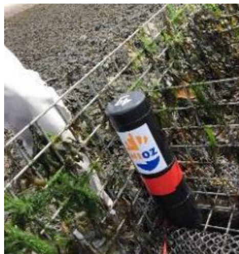
Figure 13. Wave gauge meter attached with cable ties in one of the gabions at Schelphoek.
