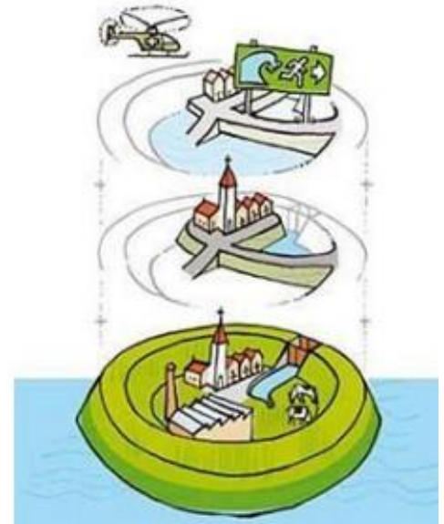
Figure 3. Multi-layer safety approach. Layer 1, prevention by dikes and storm-surge barriers. Layer 2 spatial adaptation, adapting against the changes. Layer 3, disaster management, evacuate efficiently.
