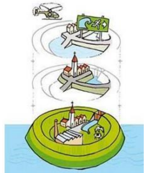
Figure 3. Multi-layer safety approach. Layer 1, prevention by dikes and storm-surge barriers. Layer 2 spatial adaptation, adapting against the changes. Layer 3, disaster management, evacuate efficiently.
