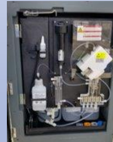
Amtax sampler measuring ammonium
