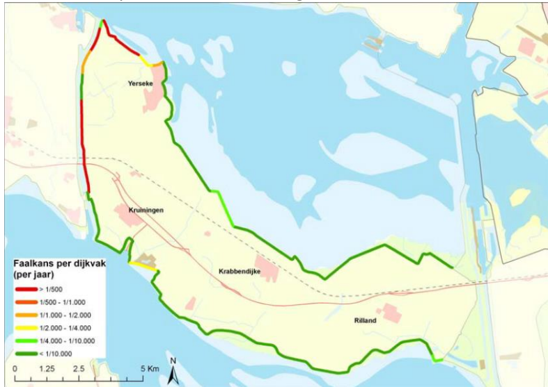
Figure 16 Failure probability of dike segments in dike ring 31 in 2011, Reimerswaal (Rijkswaterstaat, 2011)
