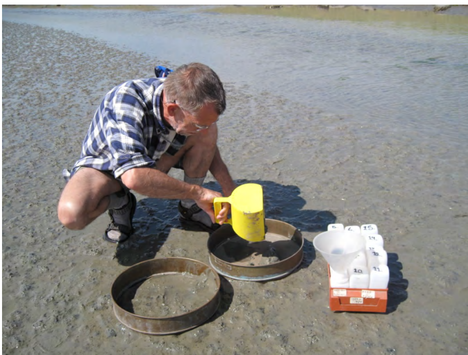
Figure 3-9- A core sampler (diameter 33 cm) was used to measure the density of the epifauna at low water. It suffices to collect the sediment from the upper few cm to collect all Carcinus and Crangon .
