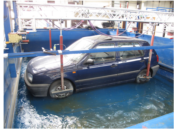
Fig. 11. Mounting of the prototype passenger car in a laboratory steel tank.
