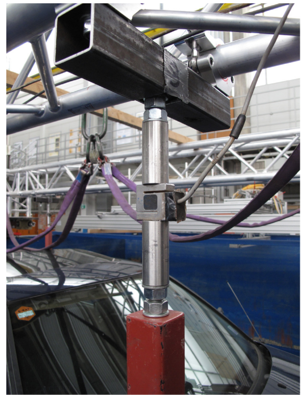
Fig. 12. Detailed view of an implemented force transducer.
