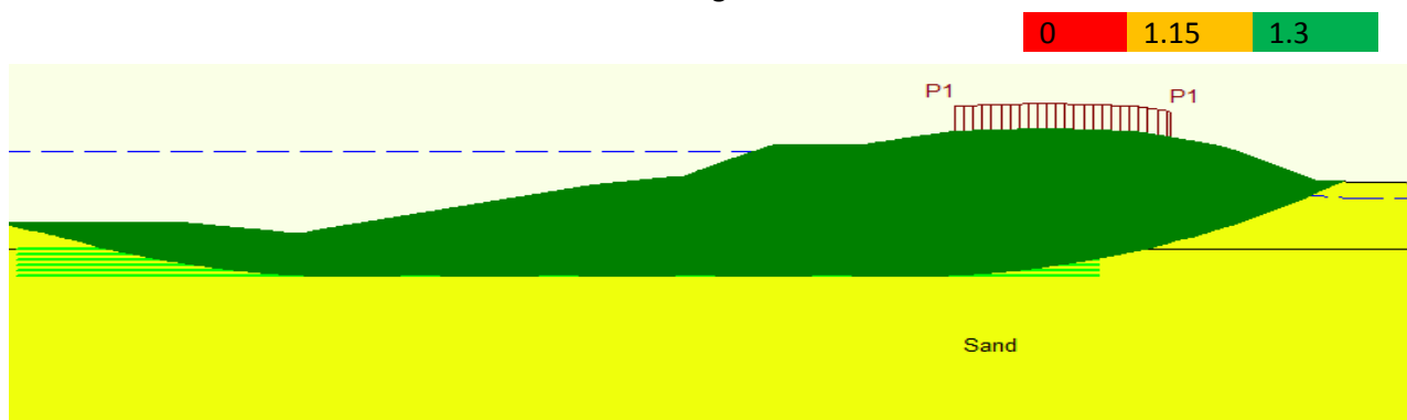
Figure 50 Slope stability overview of location three left
