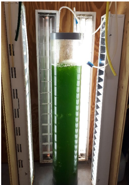
Figure 4: Bubble column containing Tetraselmis sp.
