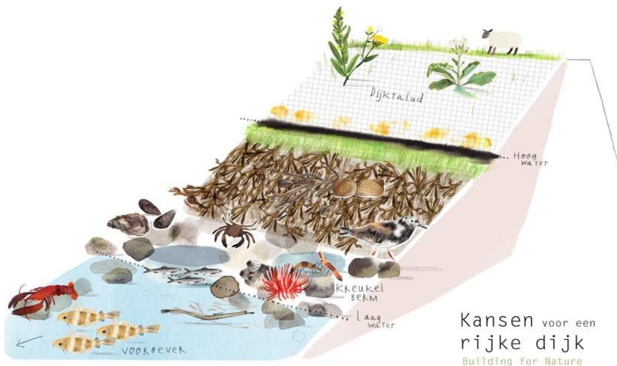
Fig. 1. An artist impression of a 'rich revetment' with a high biodiversity on the revetment, the riprap at the toe and in the foreshore.
