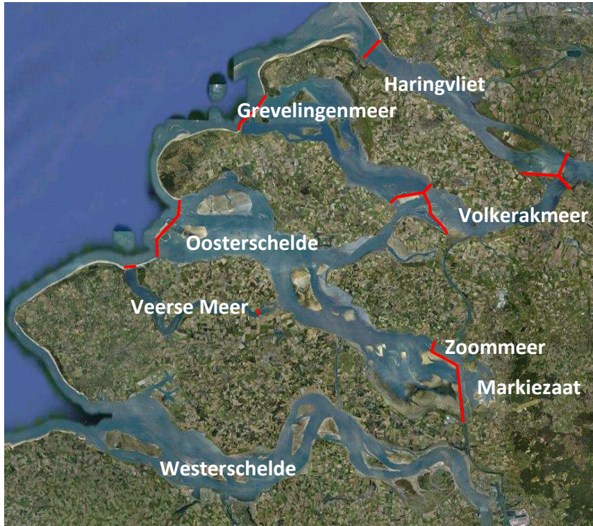
Figure 2. The South-western Delta area. Barrier dams constructed in the framework of the Delta plan are shown in red.
