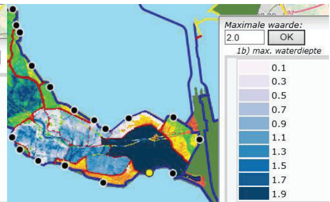
Figure 4.21: Scenario: Dike breach at Reigersbergsche Polder 1/4000. Maximum water depth in meters. (Nelen & Schuurmans, 2018)
