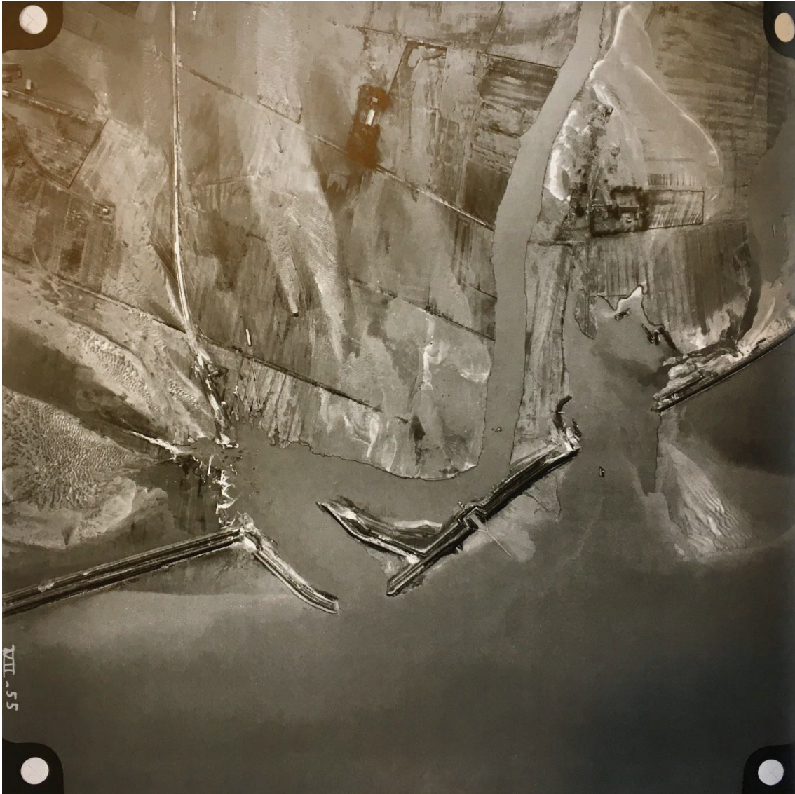
Figure 4.12: The dike breach locations at Kruiningen Veerhaven (left: 150m wide) and Oostgat (right: 200m wide). Aerial photograph taken from a Douglas DC-3 on May 1st 1953 by KLM Aerocarto, commissioned by Rijkswaterstaat. Documented in Zeeuws Archief and published by Koos Hage in his 2015 – ‘Atlas van de Watersnood 1953’ (Hage, 2015).
