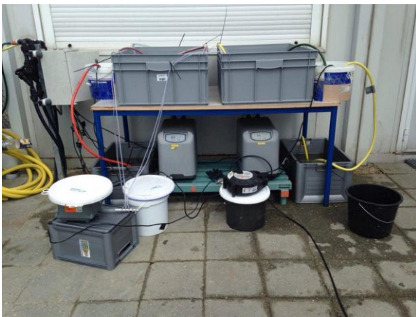
Figure 11: Experimental set-up with replicates, with flow through system, coolers, and aeration (Babaran, 2017)
