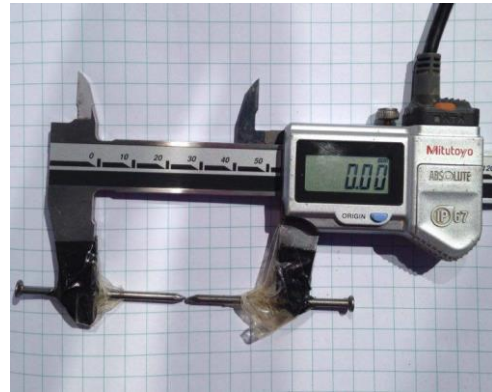
Figure 12: Vernier caliper configured to measure shell thickness (Babaran, 2017)
