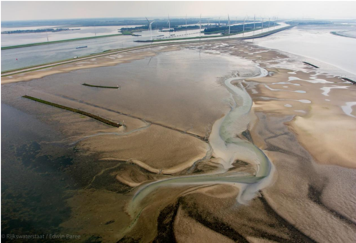
Figure 4.3 - Oyster reef around the sand nourishment; aerial picture from the north side(www.rijkswaterstaat.nl)
