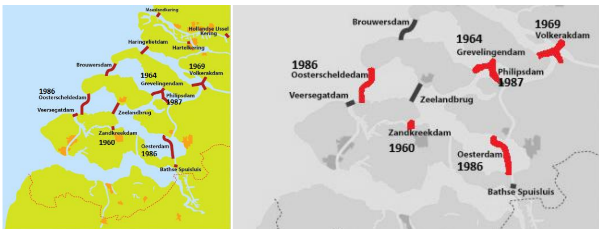
Figure 3.3 - Map of the dam realized in order to improve the hydraulic safety in the Eastern Scheldt (www.deltawerken.com)
