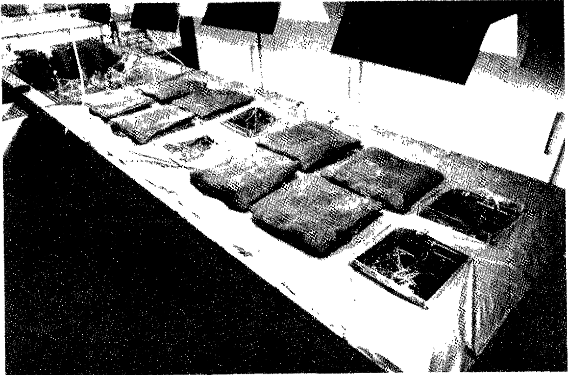
Figure 36: Aquarium experiment setup. 15 l. aquaria were cooled in a large tank, in which 18°C water flowed. Screens reduced ambient light levels (Philips daylight lamps) to the required levels.
